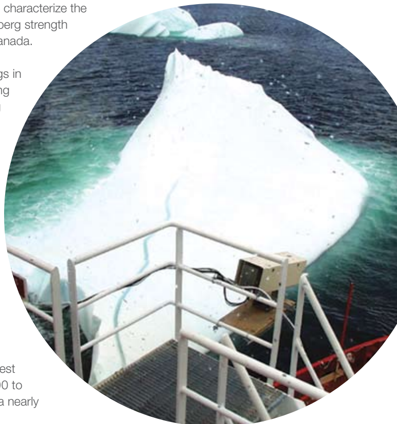
Iceberg impact tests on the Terry Fox icebreaker
