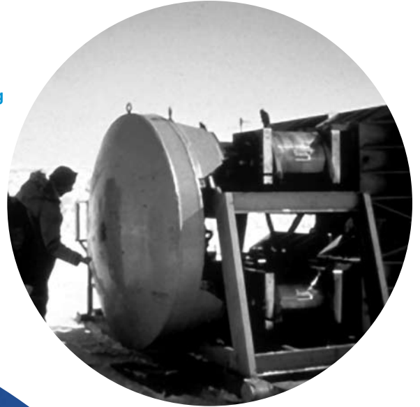
Indenter used in iceberg strength studies on grounded iceberg in Pond Inlet
