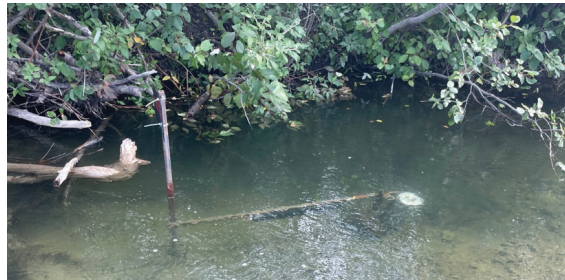
Passive water samplers deployed in the Mackenzie River
