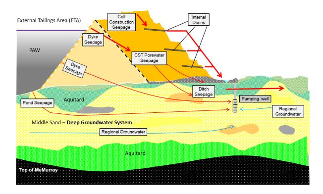
The SIS is designed to detect seepage of industrial wastewater via regular sampling and monitoring for known chemical markers. Once detected, pumping wells are activated to return the affected water to the ETA for ongoing storage and for use in the production processes. The SIS design did not account for a shallow groundwater seepage mechanism via the sand fill layer placed during construction, and therefore did not detect nor capture the industrial wastewater as it flowed off lease.
