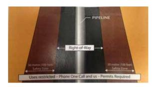
Imperial pipelines are most often located within a tract of land known as the pipeline ROW. This is a zone that allows our workers the "right-ofway" to inspect our pipelines, perform maintenance, and
