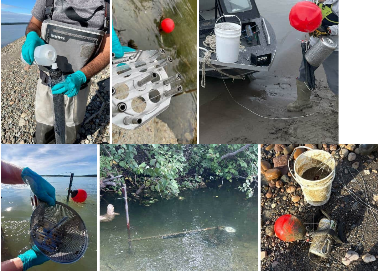
Figure 5-1: From Top Left to Bottom Right Photographs Show Examples of PDBs Being Filled with Organic Free Water; Triolein SPMD on Bracket; PSD Anchoring System for the Mackenzie River; SPMD Carrier Being Deployed Into the Mackenzie River; PSDs Deployed in Bosworth Creek; and PSDs After Being Retrieved from the Mackenzie River
